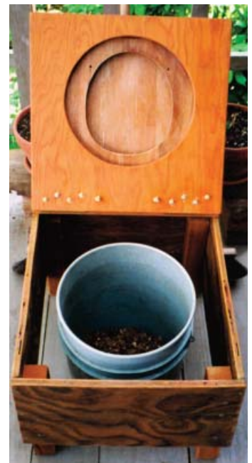
Figure 4: The toilet receptacle is easily removable.
