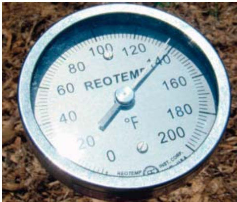
Figure 11: Temperatures measured ranged from 46C (115F) to over 74C (165F). Fluctuations varied according to size of pile, age and contents.
