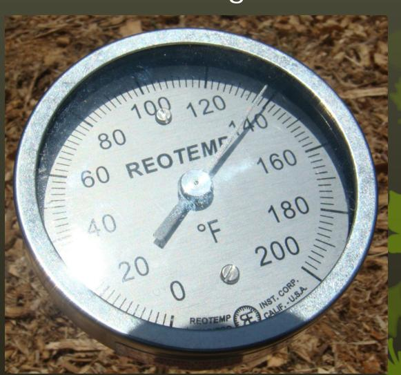
After 6 months, temperatures were still at 55C. Only 3 days at this temperature is required for pathogen elimination.
